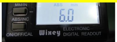
After calibration, lift the upper casting to 6" (10014) or 8" (4430) and check if the scale and DRO show the same.
