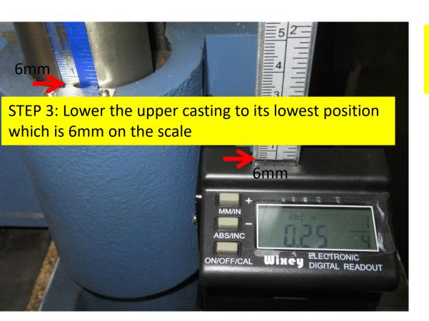
STEP 4: Loosen this screw to move the DRO to 6mm on the scale and tighten the DRO
